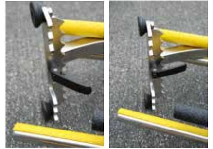
**3)** Rotate lower circle grip and set to pier or ice mode. Align pins with holes and lock lever.
