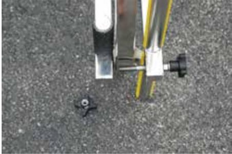
4) Locate tensioning knobs and place through holes.
