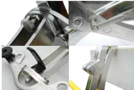
Lubricate all pins, hinges and handles with a silicone based lubricant.
