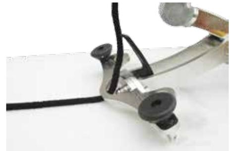
**27)** Run rope through upper grip loop and anchor away from for entry point.
