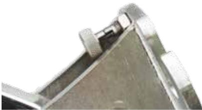
**22)** Pull pin and rotate a quarter turn to hold open.
