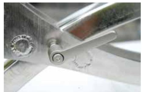
**Handle** - Pull out and rotate to re-index
