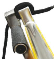
**26)** For ease of raising and lowering ladder, insert a utility rope through back hole and tie to front hole.
