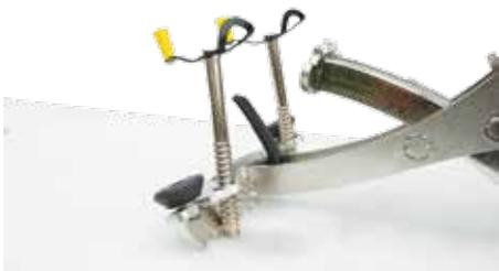
**25)** For additional safety and stability, insert ice screws in the ice screw holes.
